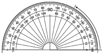
Place the centre of the protractor at one end of the arm so that the base line of the protractor lies along the arm. Find  $60^\circ$  and make a mark.
